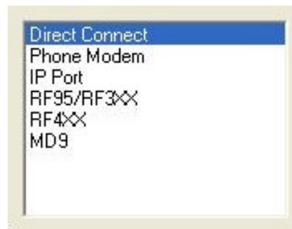
Figure 5. This dialog box shows the different modes of connection. Click on Direct connect as Default
