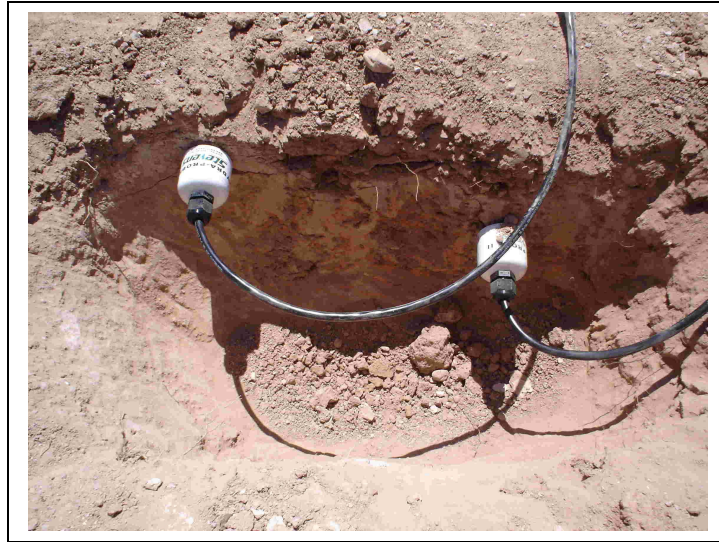
Figure 30: Vertical placement of sensors
