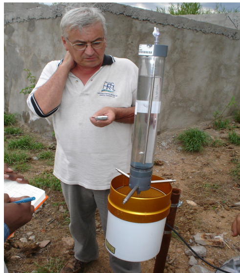
Figure 37: Setup and time measurement during the dynamic calibration procedure.
