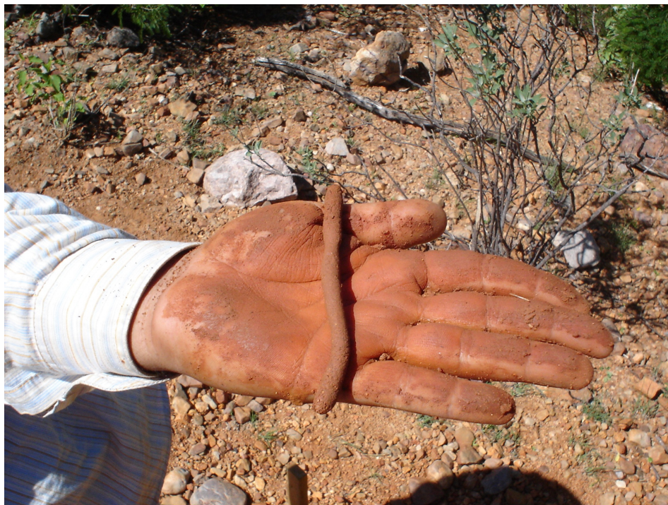
Figure 45: Example of soil plasticity: In this case soil has high plasticity (i.e., vp) and correspondingly clay content
