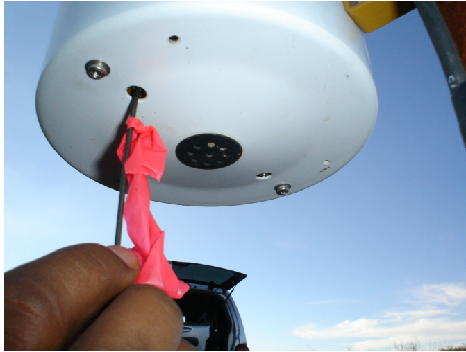
Figure 36: Adjusting the height of the pole under the bucket using an Allen wrench during the static calibration procedure
