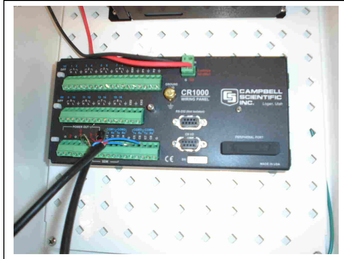
Figure 27: Solar panel connection in to the datalogger
