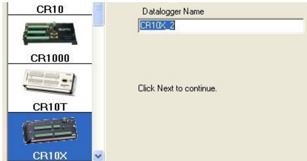
Figure 4. Datalogger models from Campbell Scientific. You need to choose CR10X, CR1000, or CR10 as the default Model
