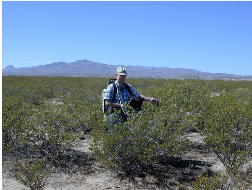
Figure 14: Example of field spectroradiometer usage. Check the shade projected by the operator. In this case, the measurement is not the optimal because the operator shadow is projected over the creosote bush, thus, can influence the reflectance or radiance readings.
