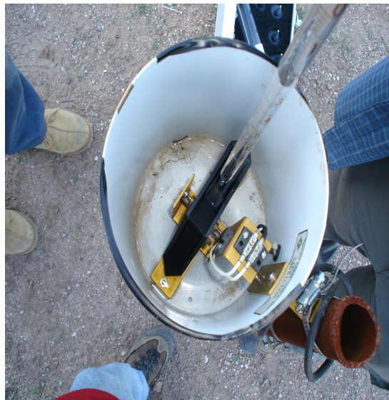
Figure 33: Burette filling a TB rain gauge bucket with water during the static calibration procedure
