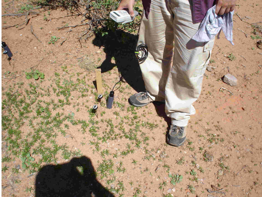
Figure 9: Soil moisture measurements using theta probe. Soil temperature is measured using thermometers at different depths.
