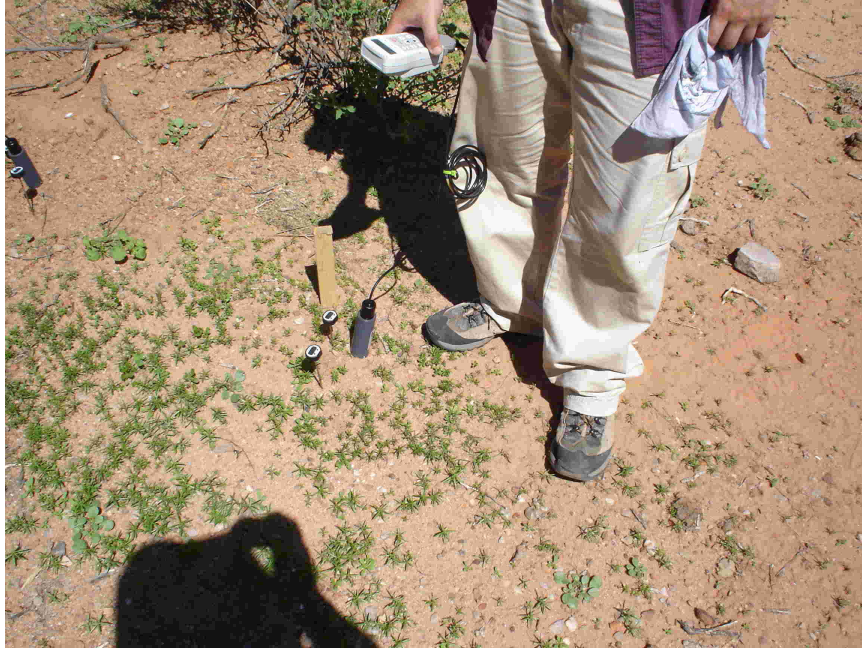
Figure 14: Soil moisture measurements using theta probe. Soil temperature is measured using thermometers at different depths.
