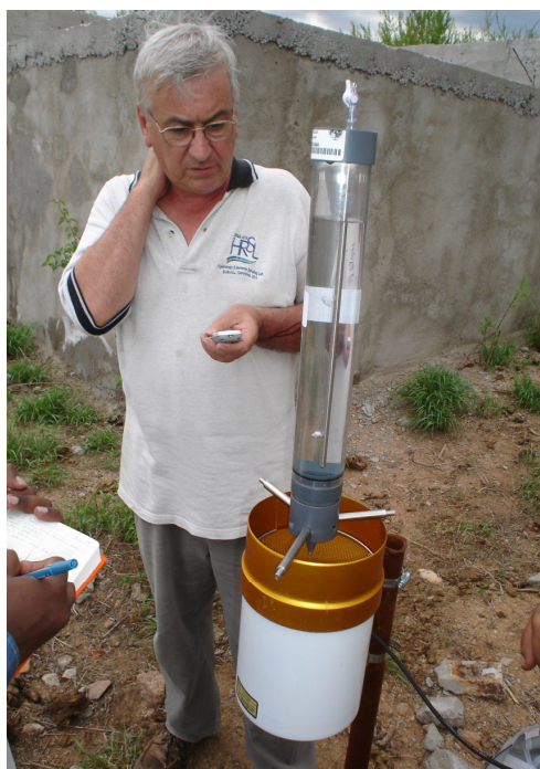
Figure 67: Setup and time measurement during the dynamic calibration procedure.
