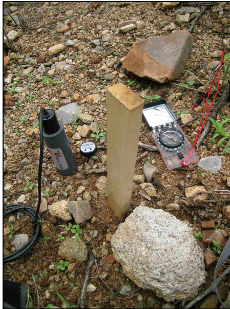
Figure 12: Some of the equipment used to estimate soil moisture and soil temperature. This includes theta-probe, thermometers, compass etc.
