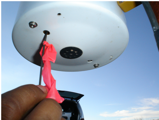
Figure 66: Adjusting the height of the pole under the bucket using an Allen wrench during the static calibration procedure
