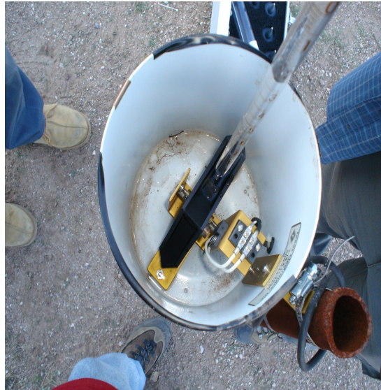
Figure 63: Burette filling a TB rain gauge bucket with water during the static calibration procedure
