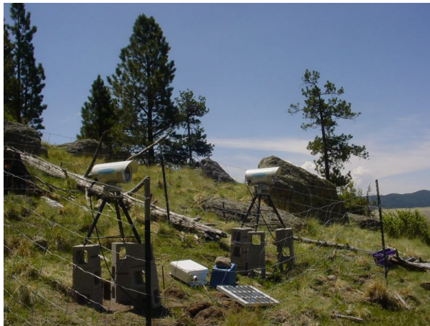
Figure 69: Two LASs (one receiver and one transmitters of two separate transects) during the LAS intercomparison study in northern New Mexico (Kleissl et al., 2008). The corresponding transmitter and receiver are 2 km away.
