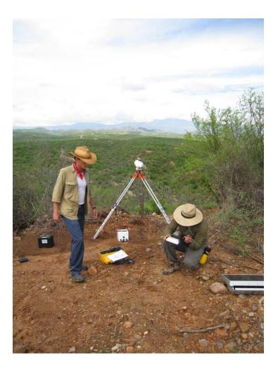
Purpose: The purpose of this project was to measure a single sensible heat flux measurement for an area on the scale of 1-3 km for comparison to calculated fluxes using satellite imagery.
