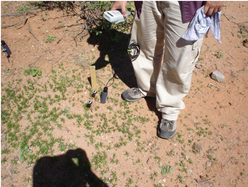
Soil temperature at 1, 5 and 10 cm depth. Soil moisture (Thetaprobe)
