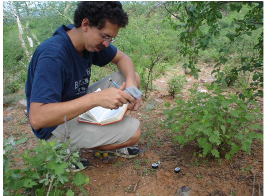
Soil surface temperature (IR thermometer)
